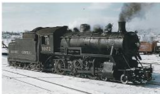
Photo Robert E. Collier Montreal Locomotive Works Canadian Pacific #1072 Class D-10k "Ten-wheeler" leased to Quebec Central at Sherbrooke - February 1960
